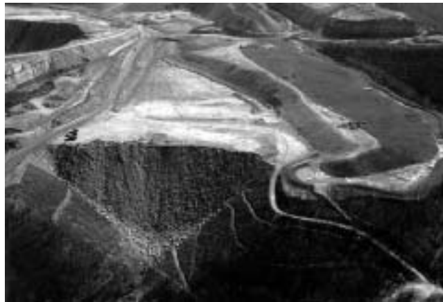
Coal companies blast off mountain peaks and push millions of tons of mining waste rubble into surrounding valleys, burying miles of streams.
