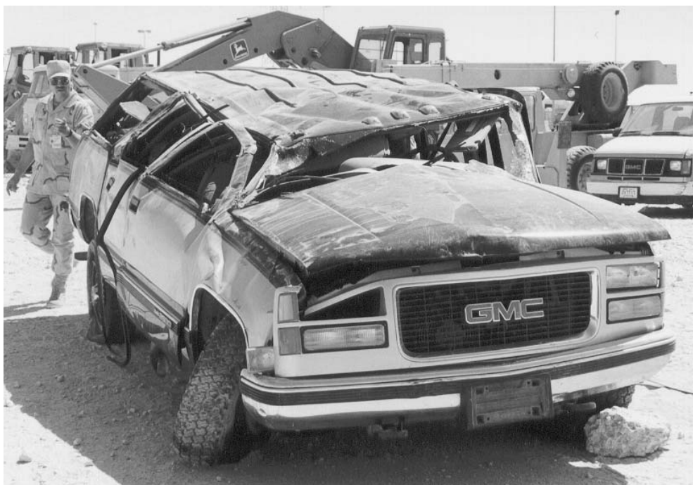
Three U.S. Air Force personnel riding in this GM Suburban were killed and three others were injured when a Goodyear tire came apart. TLPJ is battling to unseal Goodyear tire documents in this rollover case.
