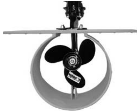
A propeller guard such as this one might save boaters from serious injury or death.
